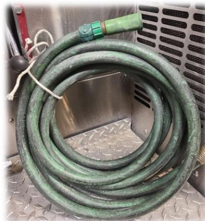
This utility hose is carried with the adapter in place
