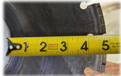
14" Blade = 4.9" max cutting depth
