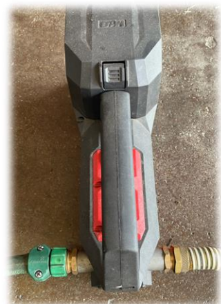
The utility hose can be connected directly to the hydrant pump
