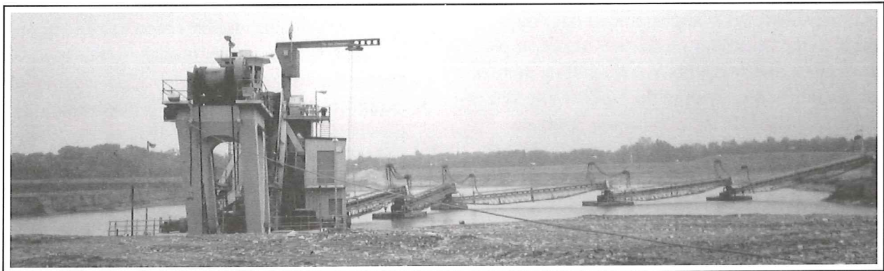
Active quarrying at the Olen Corporation, the state's largest sand and gravel operation. The dredge pictured in the photo is powered by electricity, which reduces the potential for groundwater contamination.
